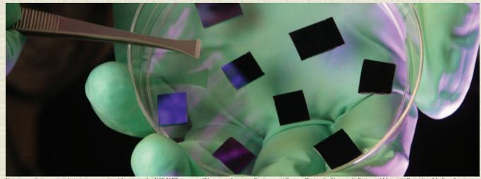
nomagnetic memory substrates are prepared for use in the NSF-NIRT program, "Nanomanufacturing Strategy and System Design for Nanoscale Patterned Magnetic Recording Medium."
