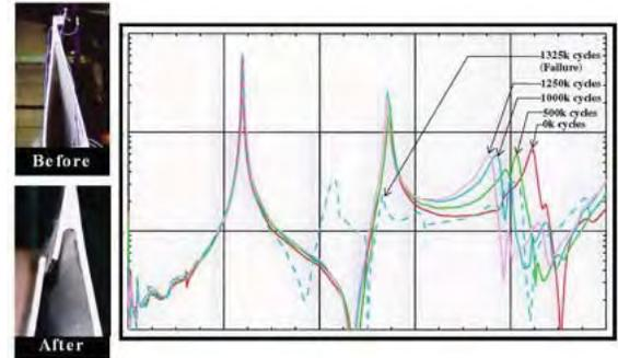
Resonant fatigue testing of blade shows torsional mode frequency "tracks" very nicely the onset of fatigue
