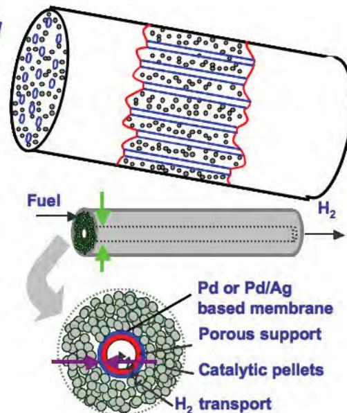
Membrane Reactor for H<sub>2</sub> Generation
