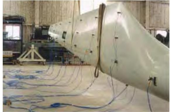
Vibration test of a blade performed in conjunction with Sandia National Laboratories at the US Department of Agriculture's Research Station in Bushland, TX.
