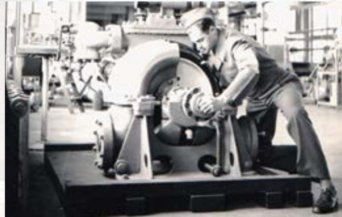
LIENHARD VISITS MIT'S THERMAL ENGINEERING LABORATORY IN 1953, AND IS INTRIGUED BY A THEN-ALREADY-OUTDATED, SINGLE-STAGE, STEAM TURBINE. PHOTO BY P. P. ROY CHAUDHURY.
