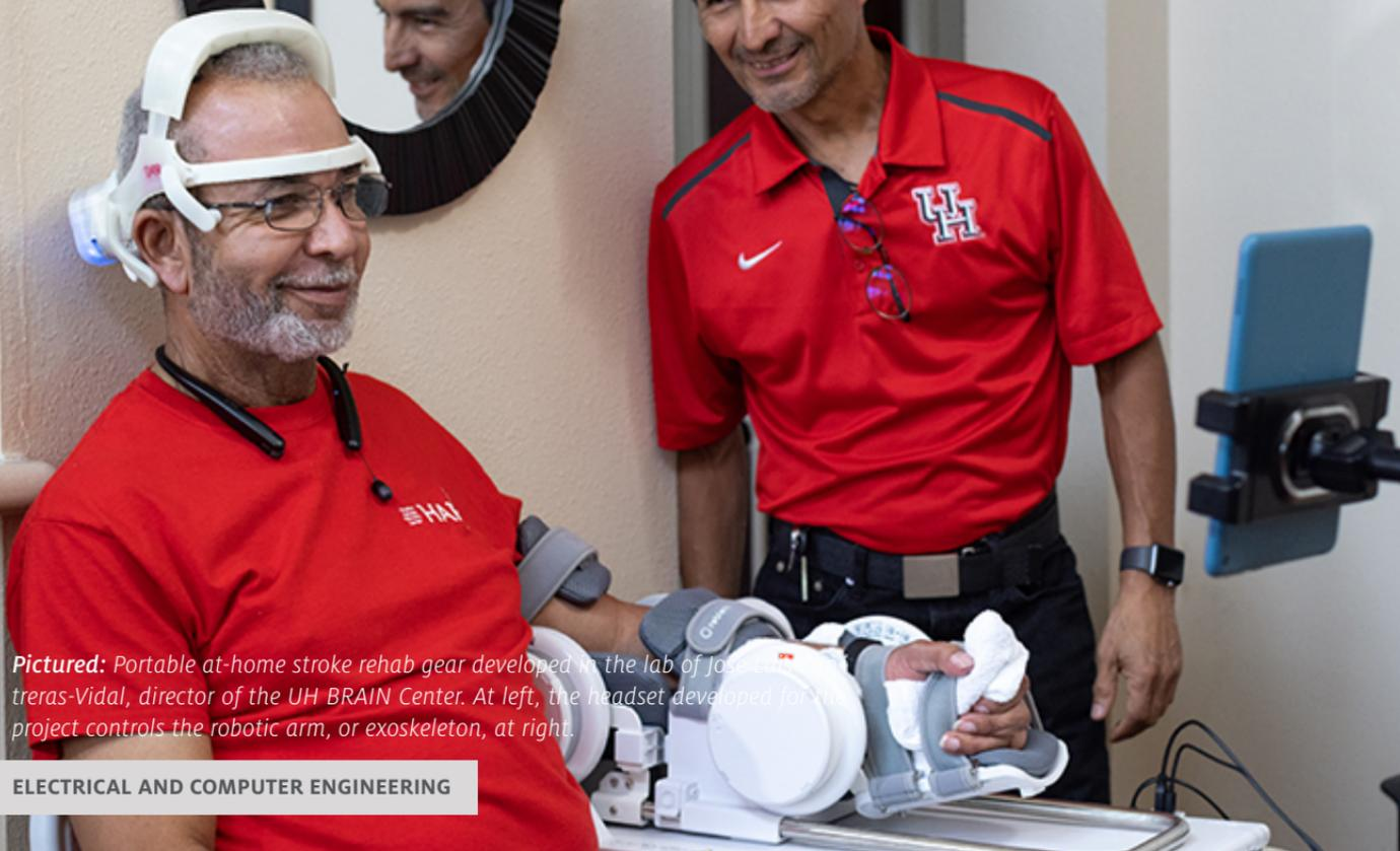
**Pictured:** Portable at-home stroke rehab gear developed in the lab of Jose Luis Contreras-Vidal, director of the UH BRAIN Center. At left, the headset developed for the project controls the robotic arm, or exoskeleton, at right.
