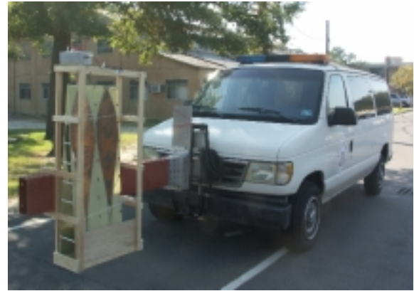
Fig. 2 Air-lunching version of the pulse GPR
