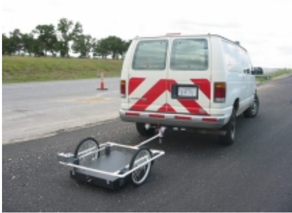
Fig. 1 Ground-coupling version of the pulse GPR
